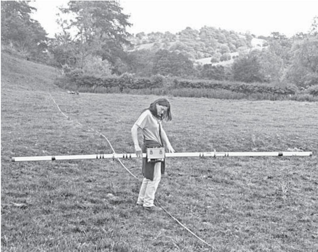
Figure 8.10 EM-31 in use in open country.
