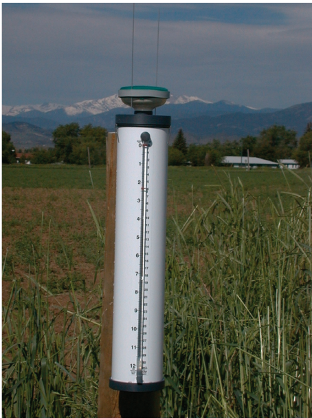
Figure 2. An atmometer installed in a field. Reference crop ET is estimated from changes in the water level, which is visible through the graduated site tube in front of the distilled water reservoir.
