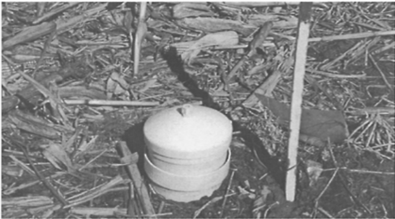
FIGURE 18.3 A static chamber is used under field conditions to assess the gaseous emission over a short period of 10 to 15 minutes. (Waterman Farm, Columbus, OH, 1998.)
