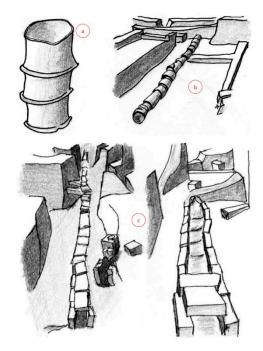
**Figure 2.** Schematic diagram of drainpipes found in Iran. (**a**) Old Elamite period (ca. 2700–1600 BC), (**b**) Protoliterary period (ca. 3400–2900 BC), and (**c**) drainage canalization made from baked clay bricks (ca. 3400–2900 BC) [35–37].
