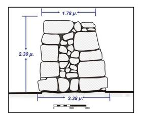
Figure 4. A schematic design of the dyke in Kopais [14].
