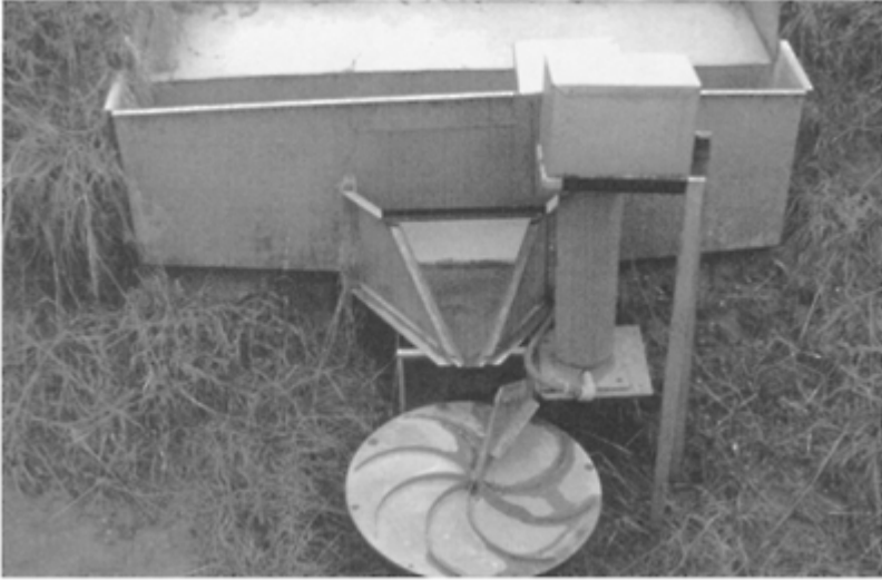
FIGURE 9.18 A Coshocton wheel sampler to obtain runoff sample.
