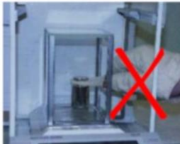
Users hand in balance enclosure affecting the thermal stability.
