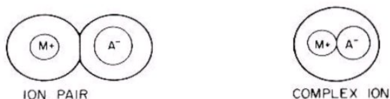
FIGURE 3.3. Diagram of an ion pair and a complex ion.
