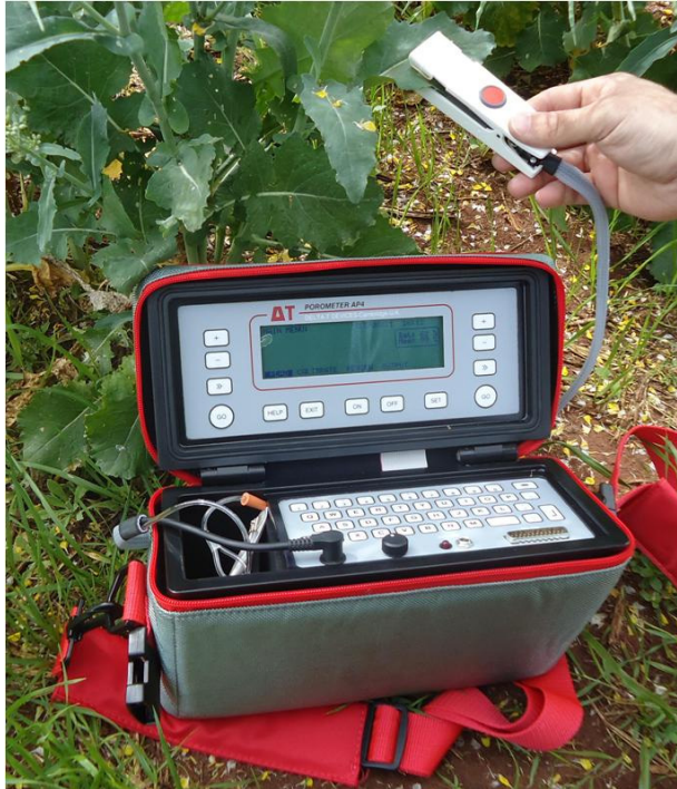
Fig. 9. Stomatal conductance determination using a porometer. Photo: Ana Cláudia Pedersen.
