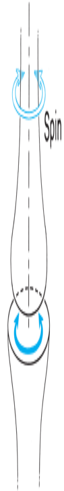
FIGURE 5.6 Representation of spinning. There is rotation of a segment about a stationary mechanical axis.
