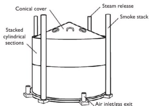
Figure 8.5 Transportable metal kiln, Tropical Products Institute (TPI)
