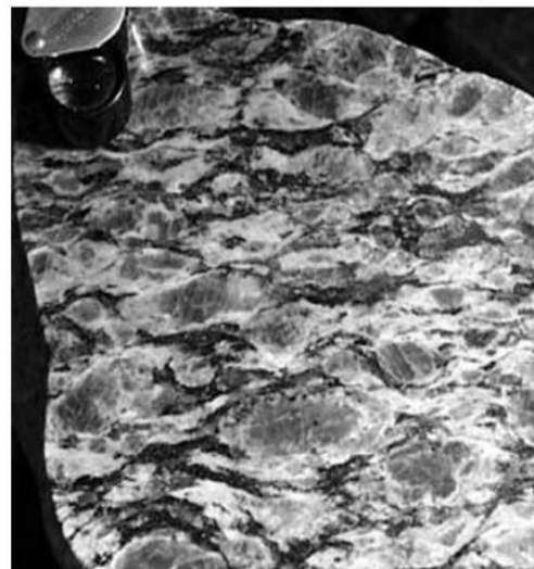
FIGURE 18 Augen gneiss with eye-shaped porphyroclasts (augen) of K-feldspar in a sheared granitic matrix.
