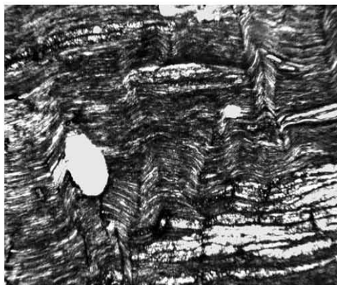
FIGURE 30 Kink bands involving cleavage in deformed chlorite. Inclusions are quartz (white), and epidote (lower right). Field of view \sim 1 mm.
