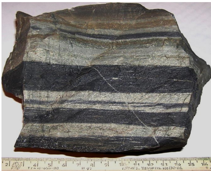
Fig. 9. Hornfels from the Novosibirsk region of Russia. The dark and light bands are bedding. The rock has been recrystallized during contact metamorphism and does not display foliation.
