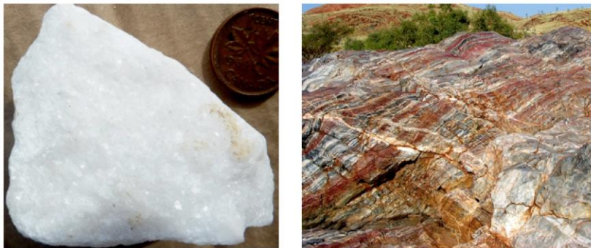
Fig. 7. Marble with visible calcite crystals (left) and an outcrop of banded marble (right)
